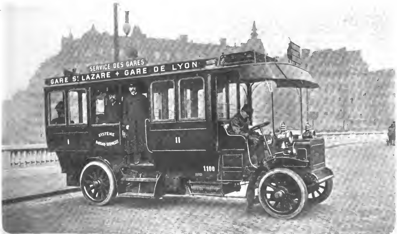
STEAM OMNIBUS WHICH HAS REPLACED HORSE SERVICE BETWEEN THE LYONS AND ST. LAZARE STATIONS IN PARIS.
